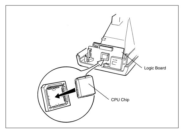
Figure 5-17 Firmware CPU
